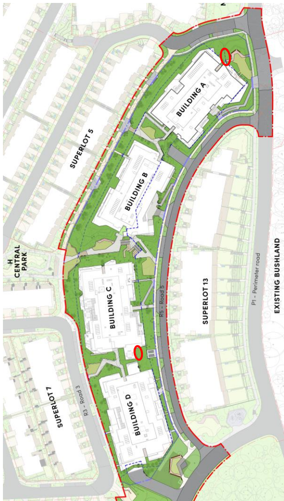
Figure 28 – Basement Exhaust Locations
