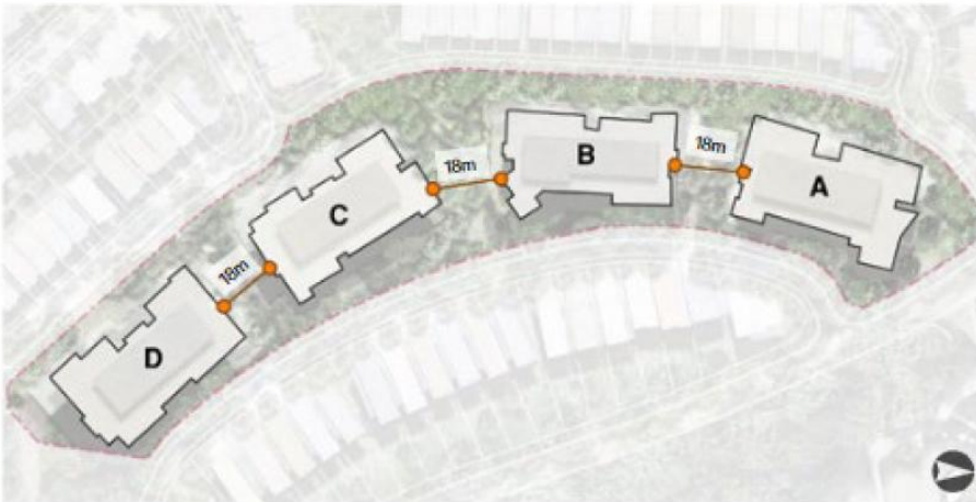
Figure 26 –Apartments Building Separation
