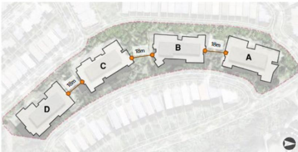
Figure 26 –Apartments Building Separation
