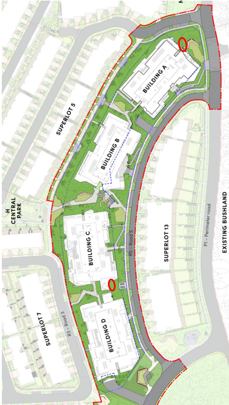
Figure 28 – Basement Exhaust Locations
