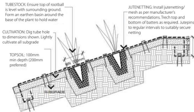
Jute netting mesh to be installed as per manufacturer's recommendations. Indicative detail shown only.
